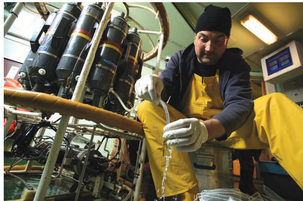
Biogeochemist Helge Niemann drains water from a rosette canister for radioactive testing of methane-loving bacteria called methanotrophs.
